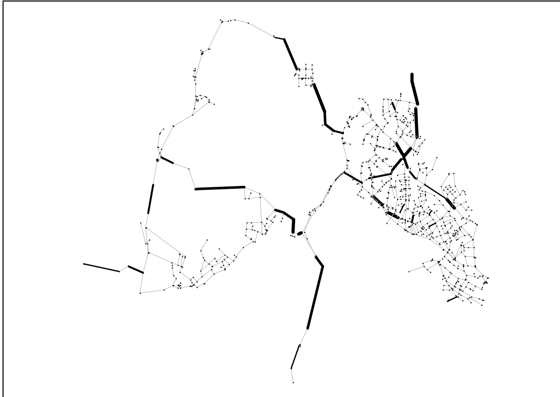
Figure 37 : Failnet-Reliab results on Crissier zone, same failure rate for all the pipes (thickness and darkness of the pipe define its importance)
