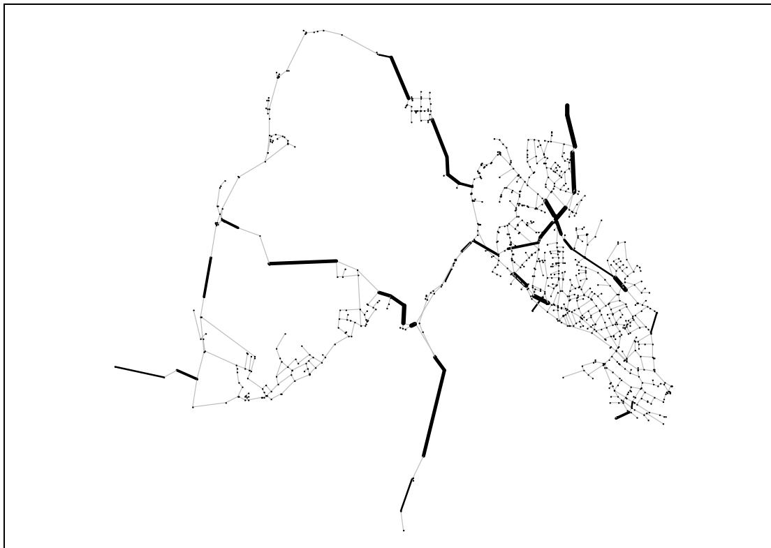
Figure 38 : Failnet-Reliab results on Crissier zone considering specific failure rates by pipe (thickness and darkness of the pipe defines its importance)
